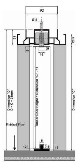
Mounting brackets MUST be recessed into doors as shown.
