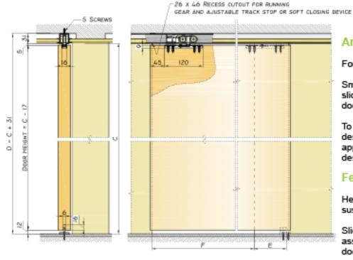
Suspension mounting plate must be RECESED into the door
